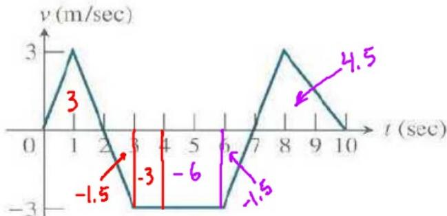
The graph of the velocity of a particle moving on the x-axis is given.
